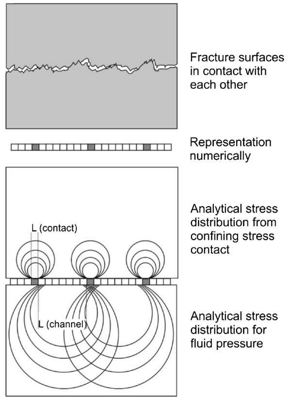
**Fig. 15.** Analytical solutions used for evaluating the impact of rock stress and fluid pressure changes.
