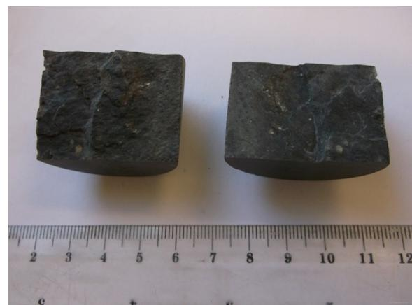
**Fig. 1.** Image of the naturally fractured sample recovered from the Wissey field.
