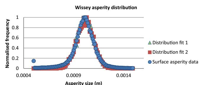
**Fig. 9.** High resolution asperity surface distribution, and two statistically identical generated profiles fitting the data.
