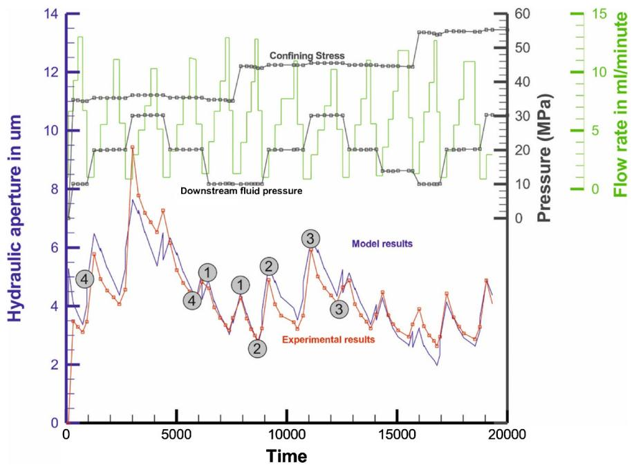
**Fig. 16.** Simulation of multiple loading cycles of confining pressure, fluid pressure and fluid flow rates. Marked points discussed in text.
