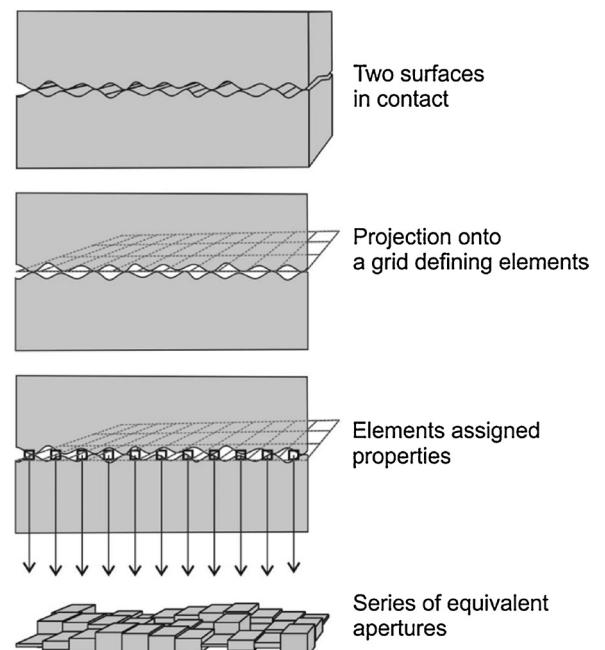
**Fig. 12.** Aperture distribution is mapped to a mesh representing the fracture plane, from McDermott et al. (2015).
