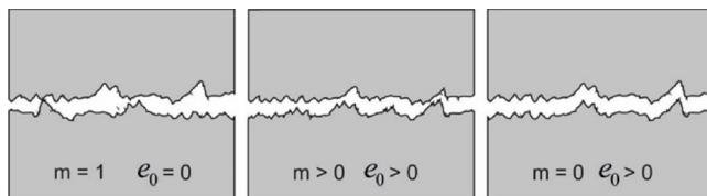
**Fig. 10.** Combination of two statistical distributions of the asperities on the fracture surface to create an aperture distribution accounting for mismatch of the surface profiles.
