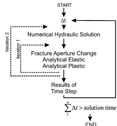
**Fig. 14.** Numerical solution procedure.
