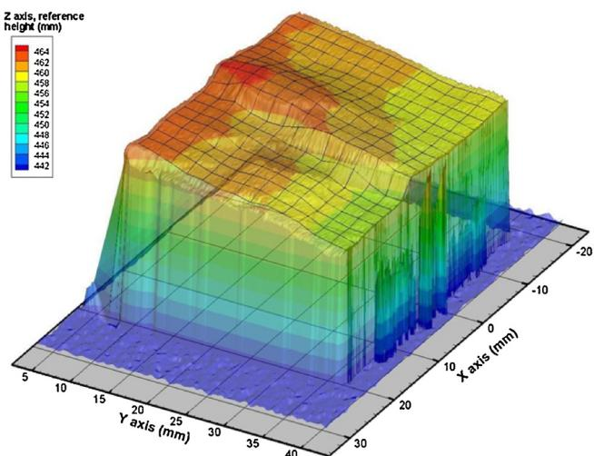
**Fig. 8.** Asperity reference surface represented as a grid.
