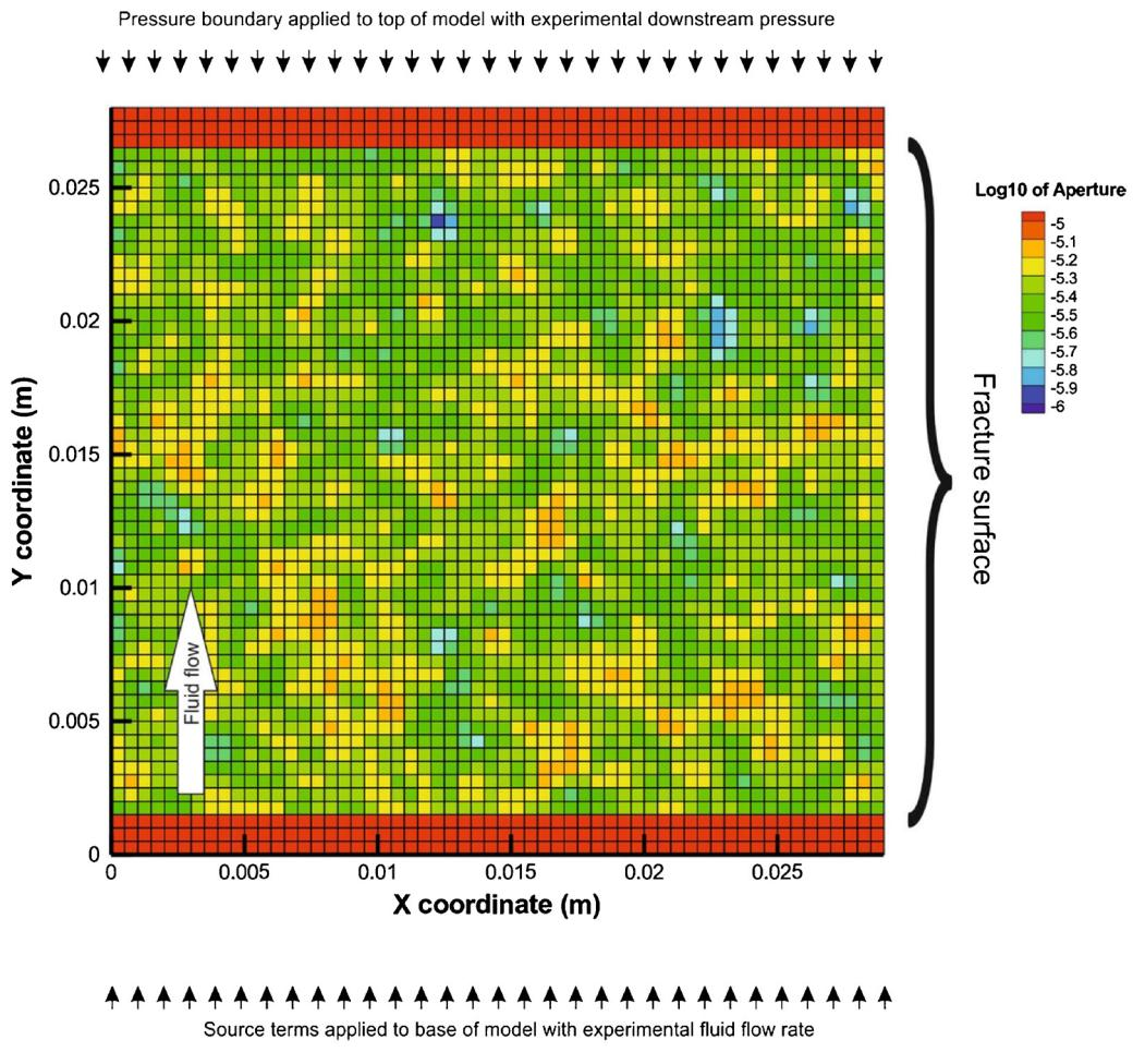
**Fig. 13.** Conceptual numerical model with discrete apertures.
