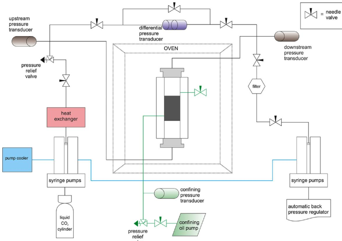
**Fig. 3.** Experimental rig schematic.
