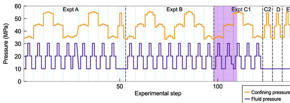
**Fig. 4.** Pressure scenarios tested and associated sample (and fluid) temperatures during flow experiments (purple band = results modelled).
