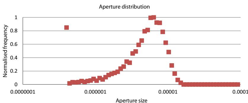
**Fig. 11.** Aperture distribution predicted from the statistical distribution of the asperity data.
