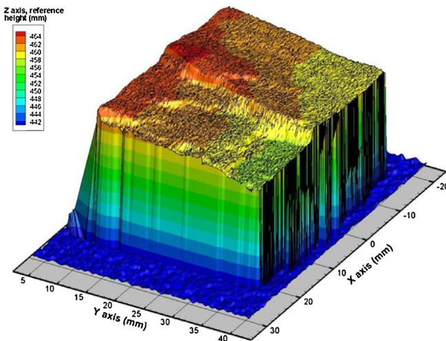
**Fig. 7.** Fracture scan data of one surface of the Wissey sample.
