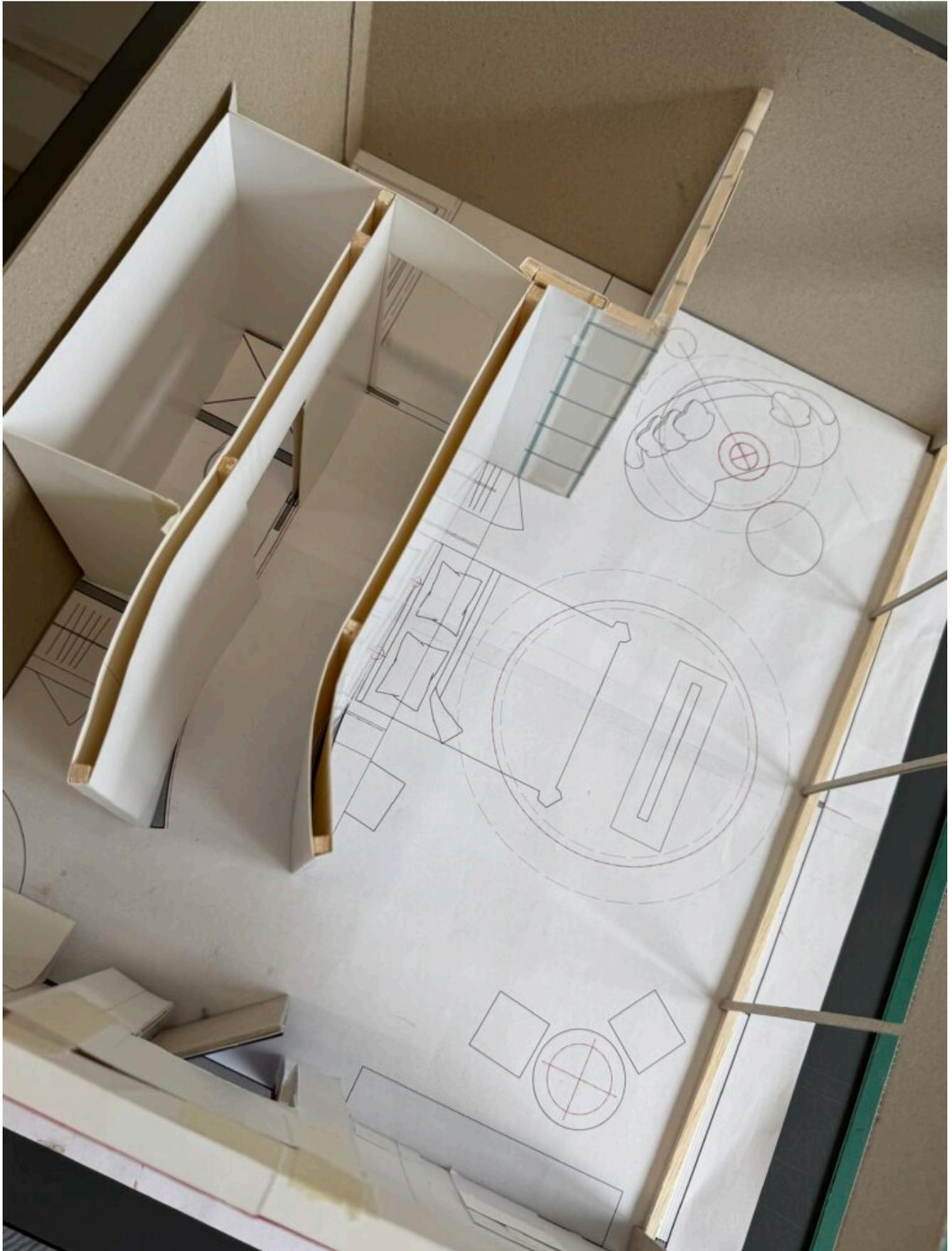
*Treating the process of building the internal walls in a similar way to framing out walls at full 1:1 scale to give the model greater stability and a sense of depth.*
