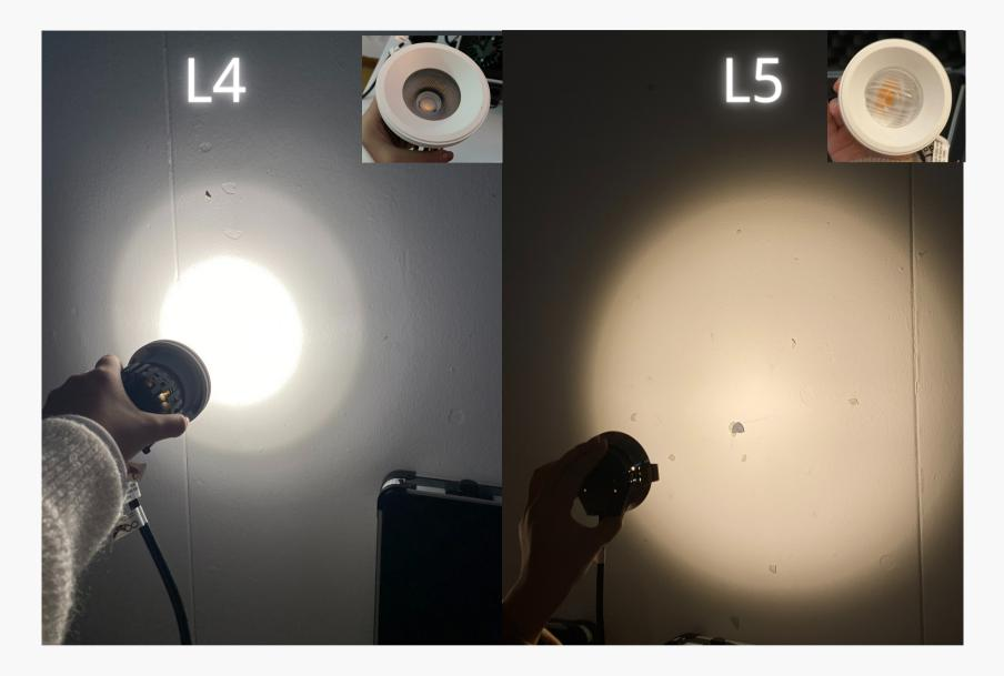
**L4:** sharp, use spread lens (cold/white color compare to L5) use aluminum reflectors, very smooth
