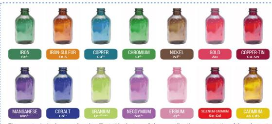
These are typical colours, and can be affected by the type of glass as well as the concentration of the colourant. Combination with other elements and compounds can also have an effect on the final colouration of the glass.
