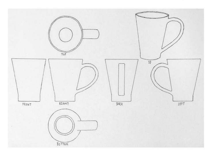
Our task this week was to draw 20 iterations of a cup. I first drew an orthographic and 3D sketch of the chosen cup, allowing me to get a better grasp of the cup's original composition.
