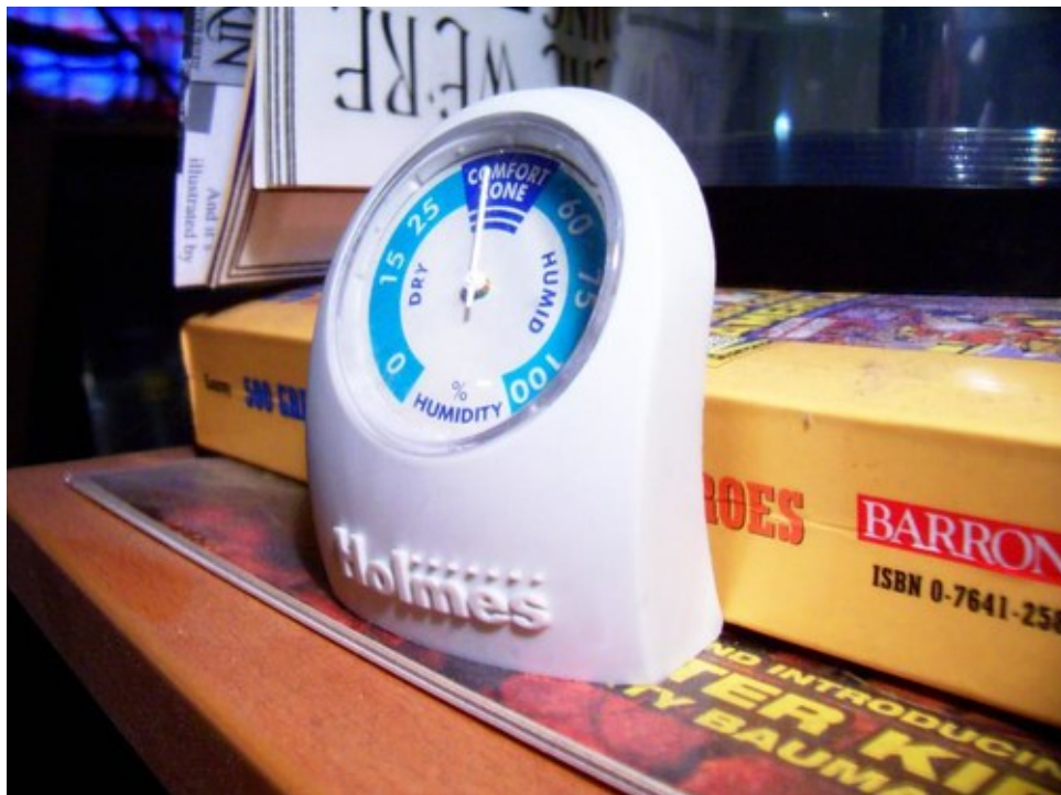
Analog Hygrometer with a region noted as "Comfort Zone". " Comfort Zone " by tmray02 , CC BY-SA 2.0 , on Openverse .
