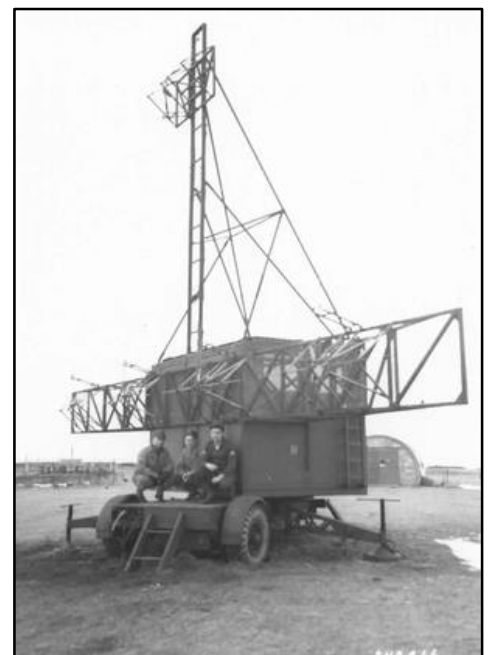
36th (Scottish) Anti-Aircraft Brigade was responsible for defending eastern Scotland. 3.7" gun deployed in 1939 and one of the two transmitter arrays of the Gun Laying radar, Mk. II.
