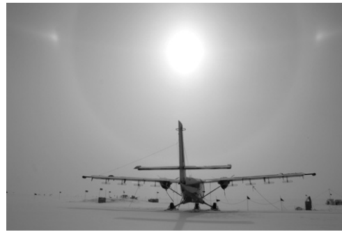
Figure 3d. Airborne radar antennae mounted on the wings of a Twin Otter aeroplane (copyright David Leatherdale).
