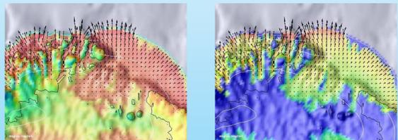
Figure 4: a) Temperatures at the ice base (red - warm, blue - cold). b) basal velocities on a log scale (blue - zero velocity, yellow - high velocities ~km/a)
