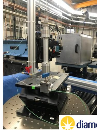
5mm  $\phi$  X-Ray hydrogen flow cell
