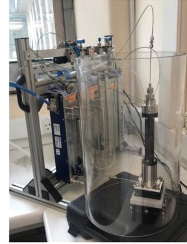
Hydrogen multiphase flow micromodel
