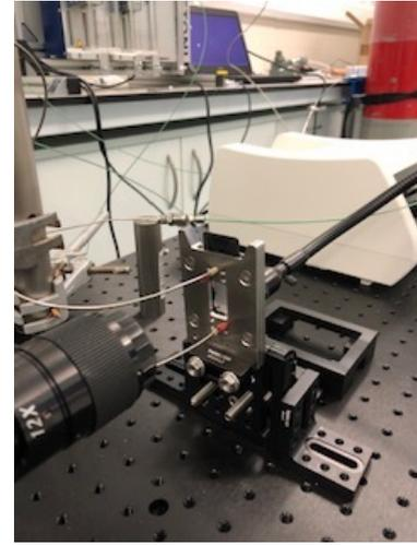
Multiphase high P/T 38mm  $\phi$  Hydrogen flow cell
