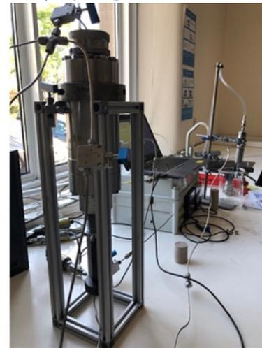
1m long, 38m  $\phi$  Hydrogen flow cell
