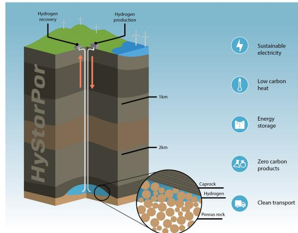
Hydrogen does not often occur naturally so, for a sustainable future, it must be manufactured by either methane gas reforming with CCS (“blue hydrogen”) or electrolysis with renewable electricity (“green hydrogen”). It can then be stored at small or large scale until it is needed.
