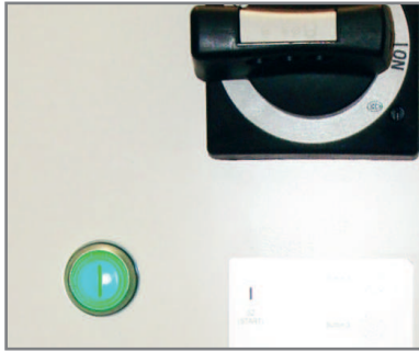
Fig. 4: S2 (Start) button below the MAIN switch
