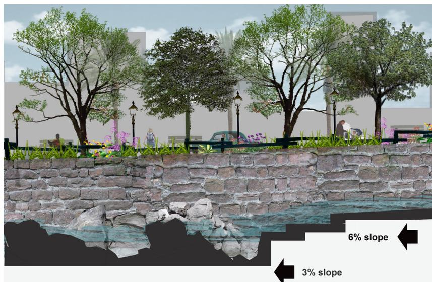
Figure 9: Photomontage (Section E). showing proposed slope modification and the use of boulders for flow control.
