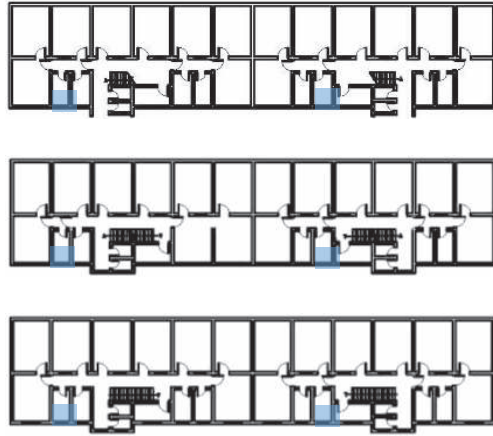
外运宿舍厕所布置 Arrangement of toilets in the apartment of foreign trade transportation fleet (draw by author) 来源：小组自绘
