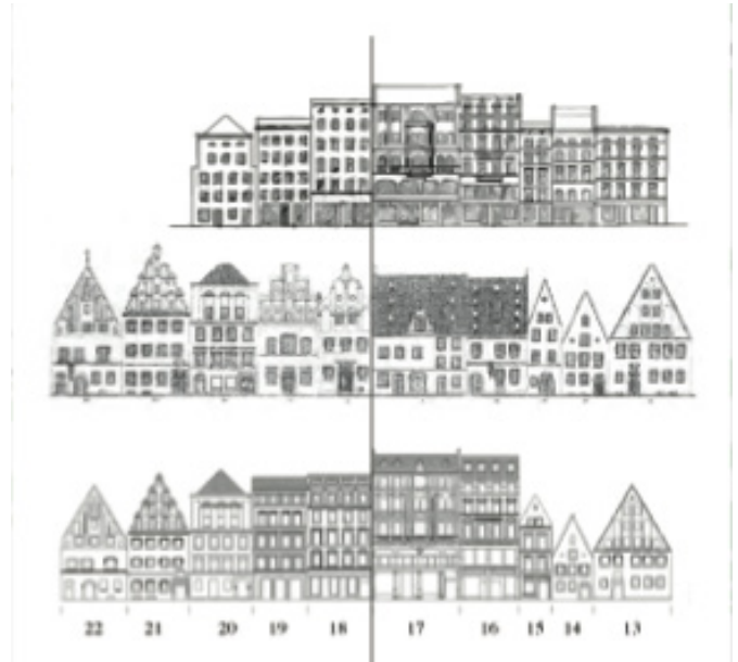
7. East Side Reconstruction drawings: TOP - 1939 Survey; CENTRE: 1950-53 Kaliski's Reconstruction Plan; BOTTOM: 2005 Siechankiewicz's Reconstruction Plan
