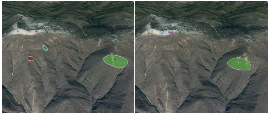
1 95% probability ellipses of locations of underground nuclear tests DPRK1–5 around Mt Mantap, North Korea, found using (left) body waves (Myers et al. 2018); (right) surface waves; overlain on topography. Green: DPRK1; blue: DPRK2; red: DPRK3; yellow: DPRK4; magenta: DPRK5. Surface-wave locations are at the mountain crests. (Google Earth)
