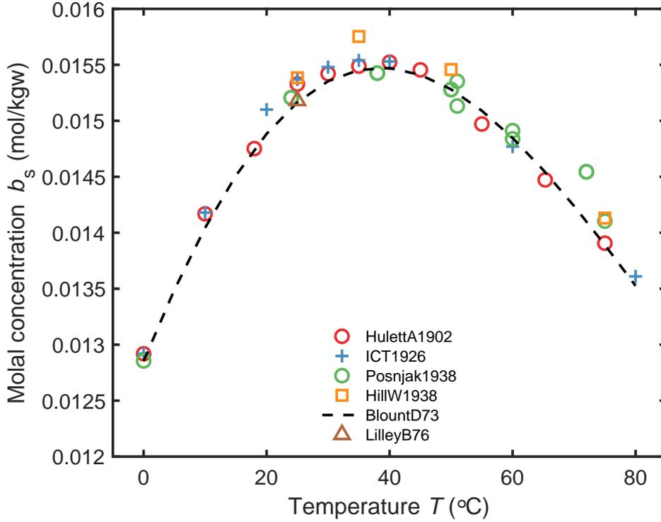
Figure 1: The measured solubility  $b_s$  (mol/kgw) of gypsum in pure water in the temperature range 0–80 °C. Data from [2, 4, 6–9]. The interpolating equation of [4] is  $\ln b = -4.354 + 0.0105T - 1.700 \times 10^{-4}T^2 + 0.584 \times 10^{-6}T^3$  at 1 atm pressure. Note that gypsum is metastable at temperatures above about 42 °C [10].
