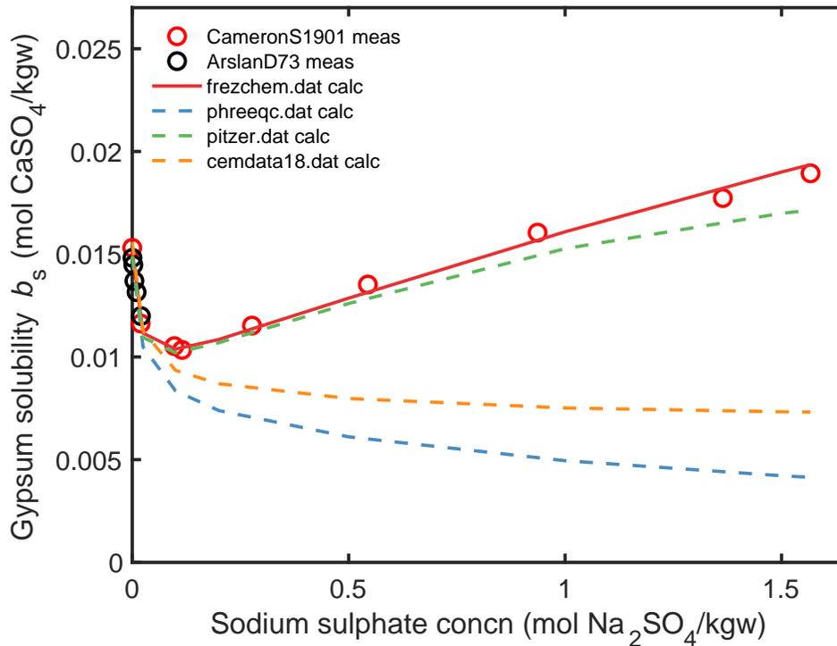
Figure 3: The calculated solubility  $b_s$  (mol/kgw) of gypsum in sodium sulphate aqueous solutions of various concentrations at 22 °C, compared with experimental data [17, 18]; the solubility of mirabilite  $\text{Na}_2\text{SO}_4 \cdot 10\text{H}_2\text{O}$  in this system is 1.567 mol  $\text{Na}_2\text{SO}_4$ /kgw.
