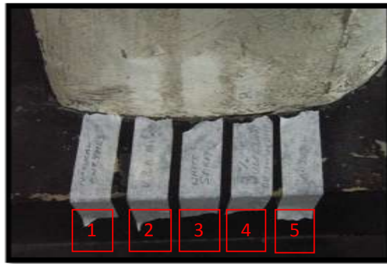
Cleaning tests with: 1 – Natural enzymes, 2 – V&A mix, 3 – White spirit, 4 – 5% Vulpex, 5 – Anjusil
