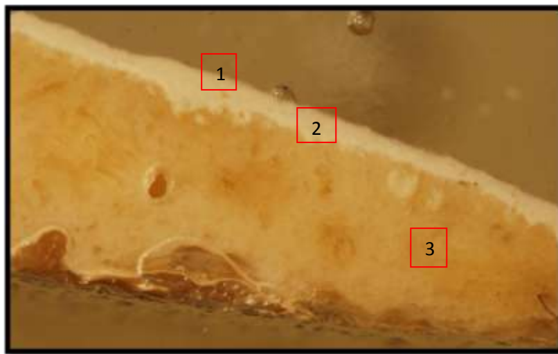
Photograph of the cross-section sample from Frieze from Temple of Athena Nike – panel 1
