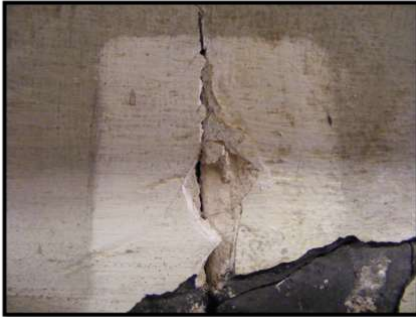
Samples of mortar were taken for analysis
